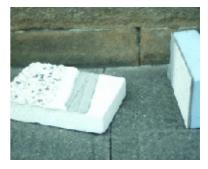
Bonded external insulation systems are difficult to recycle or re-use. Source: F. Stevenson
