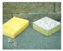
Flexible insulation bat on the left offer greater pontential for re-use. Source: F. Stevenson
